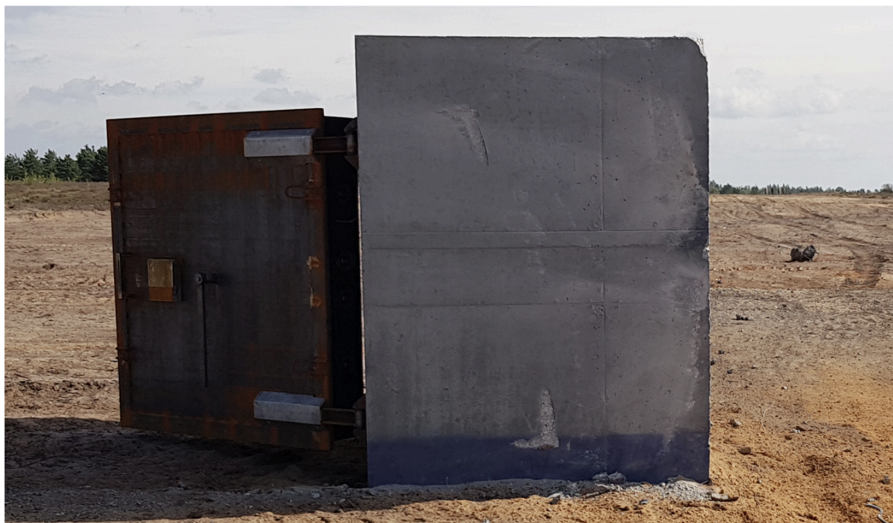
Figure 21. Test #2. Impact marks on the ES from the corner fragment of PES.
