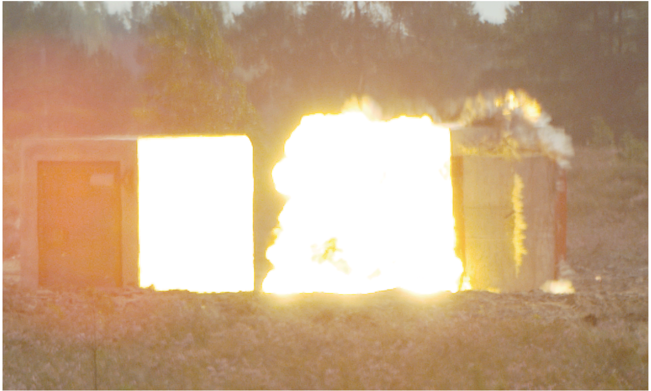
Figure 19. Test #2. Venting through the shear lines and side wall splitting vertically
