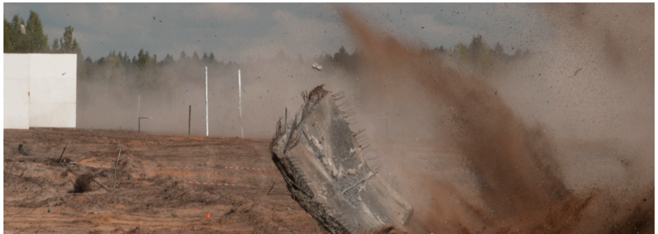
Figure 20. Test #1. Back wall rolling through the field of view of a high-speed camera facing 0° bearing to observe the left side wall fragments. Inside face towards the camera. Compression failure visible.
